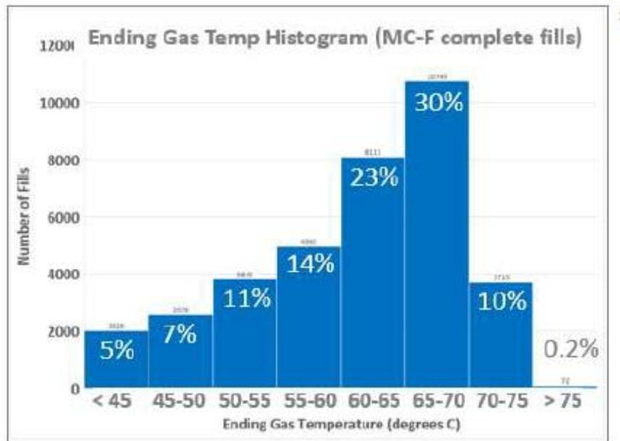
**Figure 1: End of fill temperatures for MC-Formula fills**
