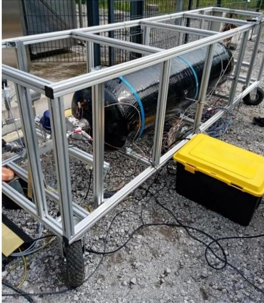
**Figure 6: Mechanical measurements on 244L vessel at ZBT**
